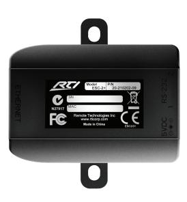
The ESC-2+ Ethernet to Serial Converter provides a convenient way to add two RS-232 ports with full two-way control capability to a system utilizing an RTI XP series control processor. Two built-in RJ-45 jacks and the included RJ-45 to DB9 adapters allow efficient cabling over standard Cat-5 wire between the ESC-2+ and the device being controlled. This allows full RS-232 control virtually anywhere there is access to an Ethernet network connection.
