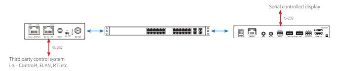
**Please note:** Only one method of RS-232 pass-through can be used at the same time. It is not possible to mix different methods of RS-232 control simultaneously.
