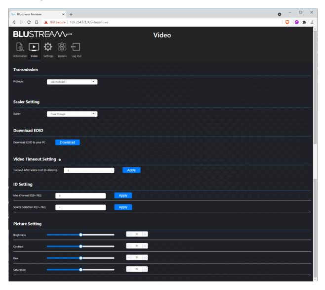
The Receiver Video Page allows you to adjust settings about the video output of the Receiver.
