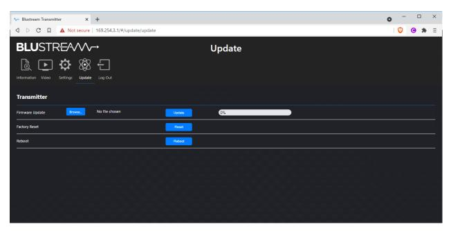
The Transmitter and Receiver Update Page allows you to update the firmware and reset the Transmitter or Receiver.
