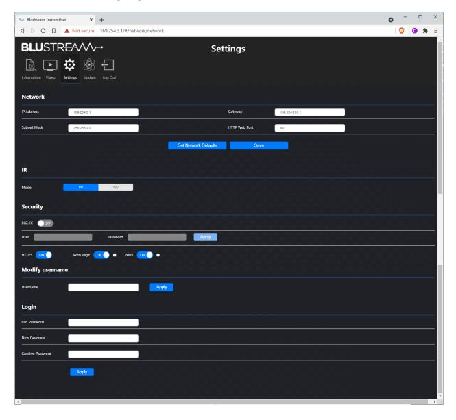
The Transmitter and Receiver Settings Page allows you to adjust settings about the network and security of the Transmitter.
