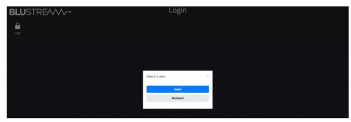
**Please note:** the first time the Administrator logs into the web-GUI of the WMF72, the default password must be changed to a unique password. Please retain this password for future use. Forgetting the password will mean having to factory reset the unit, losing all configuration settings.
