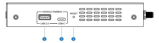
• USB-A dongle pairing port: used to pair the WMF-HDMI-D dongle with the WMF72 hub (USB connection only required for pairing). The WMF72 video output will display information regarding the automatic pairing and firmware update process.
