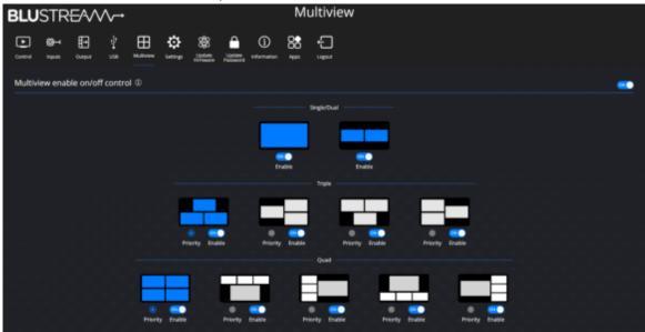
Multiview enable ON/OFF control enables or disables the multiview layout selection within the Control page. When enabled a user can manually change the layout via the Control page. When disabled, this function is removed for the user however multiview can still function if Auto mode is enabled.
