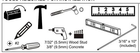
Hardware Required - not included (for installation into steel stud walls)
