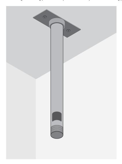
3. Thread the VESA bracket onto the pole.
