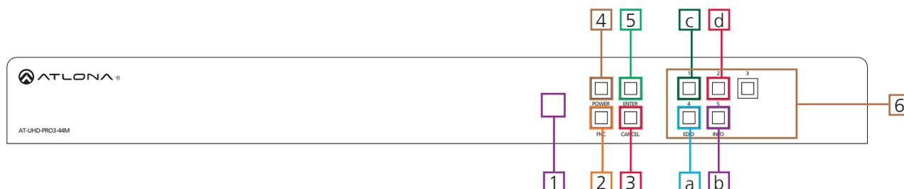
1. IR Receiver Window - Receives the signal from the included IR hand held remote control or 3rd party controller
