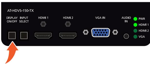
5. While pressing the **DISPLAY ON/OFF** button, connect the USB cable from the computer to the **FW** port on the AT-HDVS-150-TX.
