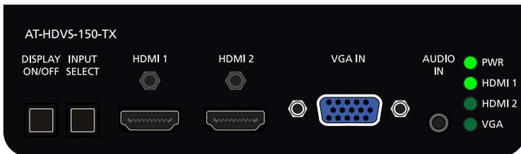
2. Press the **INPUT SELECT** button, to select HDMI 2. The **HDMI 2** LED indicator will turn bright green.
