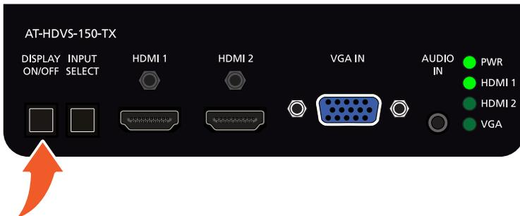
2. The power state of the display, which is connected to the receiver, will be toggled.
